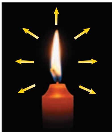
Figure 1 A light source, like a candle, sends out light rays in all directions.
